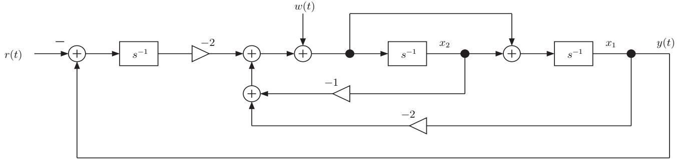
$$b) \begin{bmatrix} 0 & 1 & 0 \end{bmatrix} \begin{bmatrix} s & \boxed{-1} & 0 \\ 2 & s+2 & 0 \\ 2 & 2 & s+1 \end{bmatrix}^{-1} \begin{bmatrix} -1 \\ 0 \\ 0 \end{bmatrix} = \frac{2(s+1)}{s^3 + 3s^2 + 4s + 2} = \frac{2}{s^2 + 2s + 2}$$
