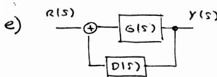
$$\frac{Y(s)}{R(s)} = \frac{G(s)}{1 - G(s)D(s)} = \frac{\frac{s}{s^2 + 2s + 2}}{1 - \frac{s(2s-2)}{(s^2 + 2s + 2)(s+8)}} = \frac{s(s+8)}{s^3 + 2s^2 + 2s + 8s^2 + 16s + 16 - 2s^2 + 2s}$$
